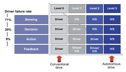
Fig. 1. Classification of the intelligent vehicle systems
