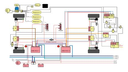
Fig. 4. 2E brake-by-wire architecture
