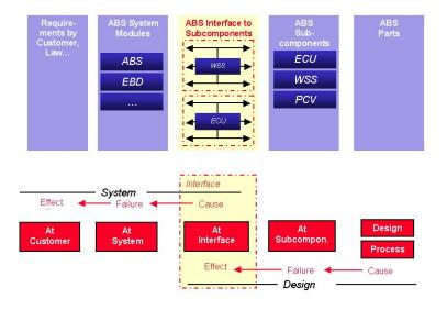
Fig. 7. Representation of the levels involved in System and Design FMEAs, with defined interfaces [4]
