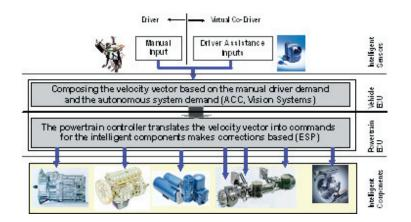
*Fig. 3. Analogue vehicle control structure to the airplane systems (PEIT project)*
